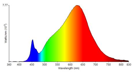
Testing was performed in accordance with LM-79-08.
